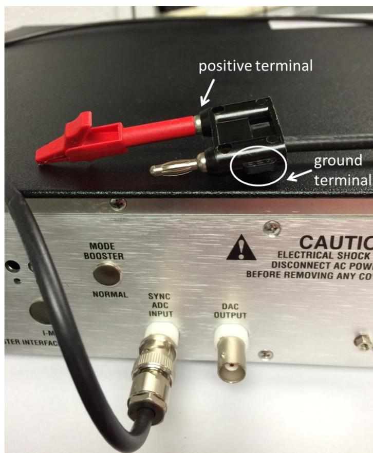
**Figure 2: Image showing how to connect between the SYNC ADC and the counter electrode using a coaxial BNC cable and BNC to double banana adapter with a single alligator clip.**
