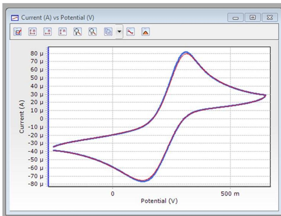
**Figure 3: Cyclic voltammetry of a Au electrode ((2 mm ± 0.2mm diameter) in 1 mM  $K_3[Fe(CN)_6]$  in 0.1 M KCl using a Pt counter electrode with (red) and without (blue) a frit. Scan rate = 200 mV/s.**
