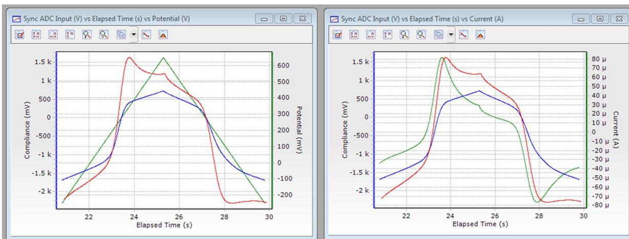
**Figure 4: Plots of the compliance and polarization potential as a function of time and the compliance and current as a function of time corresponding to the CVs in Figure 3 using a Pt counter electrode with (red) and without (blue) a frit.**
