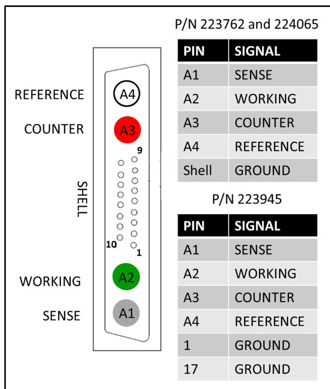
Figure 1: Pinout diagram for standard cell cables compatible with all VersaSTATs, the PARSTAT 4000, the PARSTAT MC-1000 and 500. (P/N 223762, 224065, 223945).
