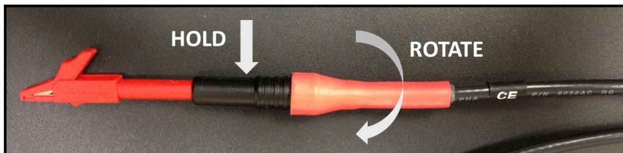
Figure 2: Image showing how to check the integrity of any standard cell cable leads.
