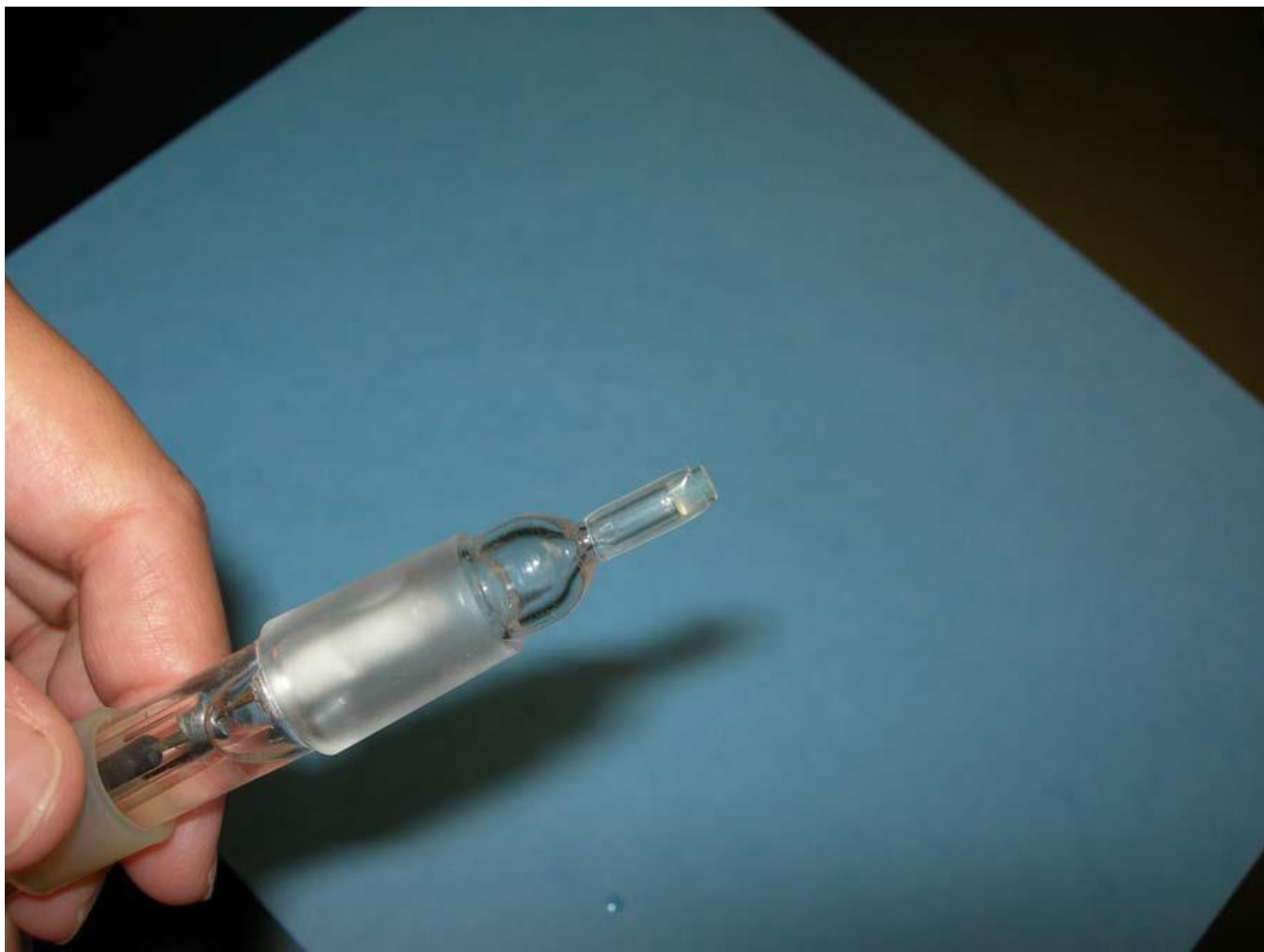
Figure 6: Slide the tubing back down over the frit, exposing the one end. If the tubing was cut to the correct length, it should be just below the top 25% of the frit's length.
