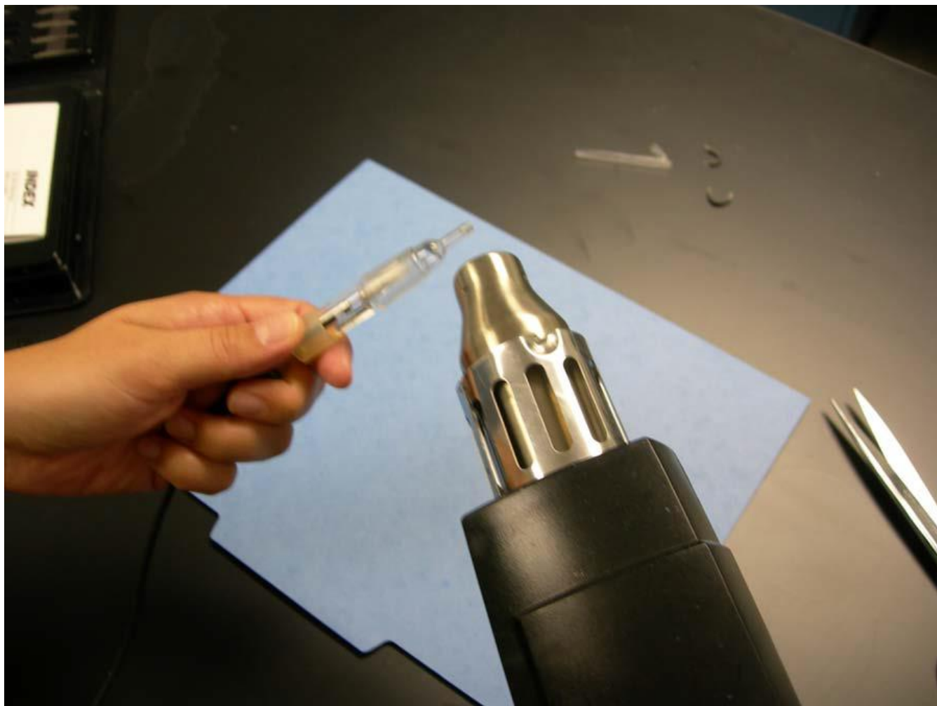
Figure 7: Heat the heat shrink tubing evenly on all sides with a hot air stream from a heat gun. The tubing will go from translucent to transparent as it shrinks around the frit, holding it firmly against the glass tubing to form a leak-tight seal. Note: If filling solution was still inside the electrode, do not invert the electrode until the glass has cooled to the touch.
