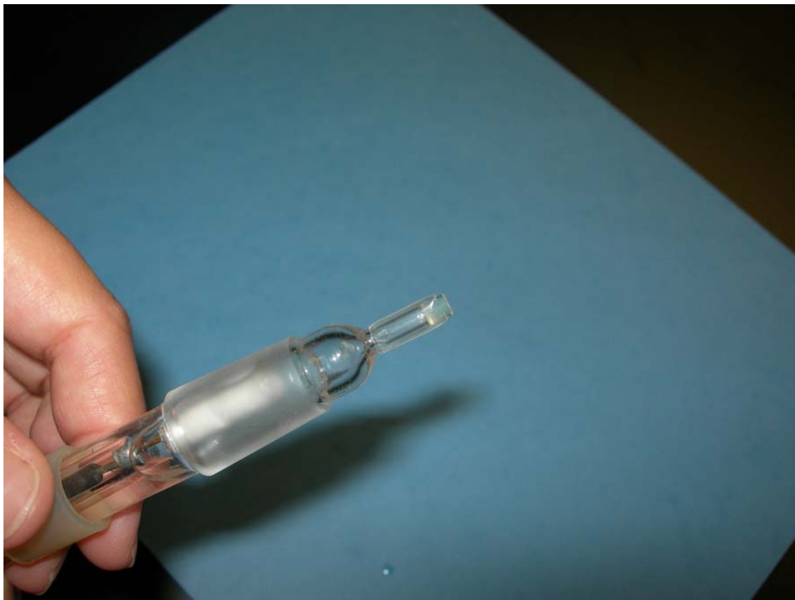
Fig. 6: Slide the tubing back down over the frit, exposing the one end. If the tubing was cut to the correct length, it should be just below the top 25% of the frits length.
