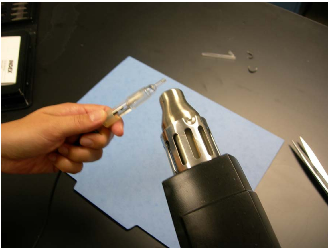
Fig. 7: Heat the Teflon tubing on all sides with a hot air stream from a heat gun. The tubing will go from translucent to transparent as it shrinks around the frit, holding it firmly against the glass tubing to form a leak-tight seal. Note: If filling solution was still inside the electrode, do not invert the electrode until the glass has cooled to the touch.
