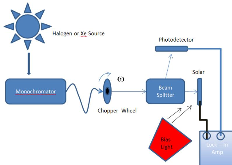
Figure 1: Typical Setup for IPCE system
