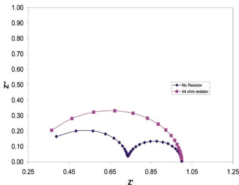
The effect of series resistor upon the impedance response of a simple resistor-capacitor network. Experimental conditions, DC load = 3Amps, AC stimulus = 10mA, frequency range = 125kHz to 1Hz in galvanostatic impedance mode.
