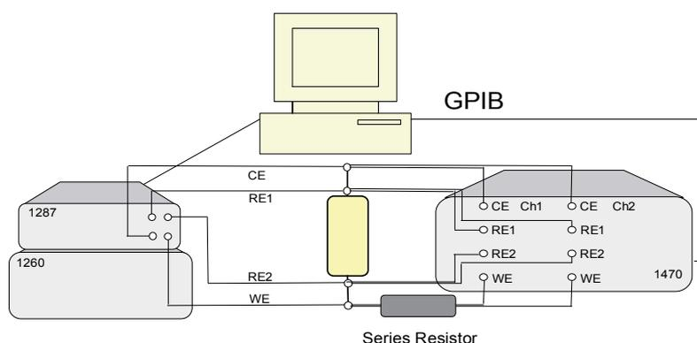
The inclusion of the resistor in the DC current loop obviates stray AC current.
