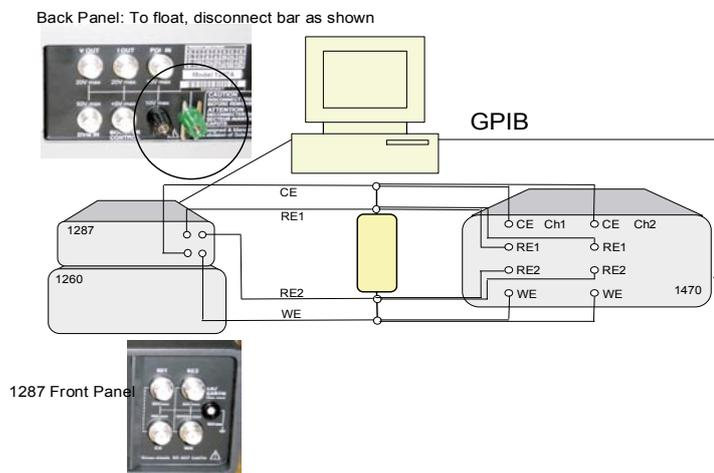
*Experimental set-up enabling high frequency, high current measurements. We recommend that all measurements should be performed with four terminal connections as shown in the diagram as this will minimise any impedance artefacts associated with cable impedance.*
