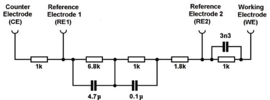
Firstly, the impedance spectrum was measured using a 1287 and 1260 at open circuit with a 10mA AC current level. Two time constants are clearly shown in figure 9 and the analysis of the curves yielded the correct values. Following this, the experiment was configured as described in the first example and one can clearly see three time constants in the impedance results when presented on a complex plane diagram.
