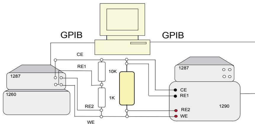
Modification of figure 1 including potential divider circuit allowing impedance studies of high voltage cells. A 1287 in conjunction with a 1290 power booster can also provide the load offering a maximum capability of 25Amps, 50V, though the compliance range of the 1287 would limit this to 30V maximum.
