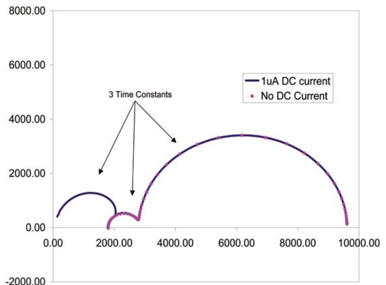
In principle all of the AC measuring current should flow through the cell. However, in practice some of the current is diverted into the DC current loop as illustrated in figure 10. All electronic loads exhibit associated capacitance and it is this that appears as the artefact at high frequencies. According to equation (1), the current flowing through the electronic load is a function of the reactance ( $X_c$ ) of the capacitance on its outputs (equation 2)
