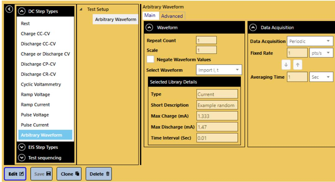
Alternatively, comprehensive Test Sequences can be set up that use more than one waveform profile together with standard CC-CV charge steps, rests, and EIS impedance analysis to monitor the effect of the cycled profiles. This example shows cycling of multiple tests in sequence:
