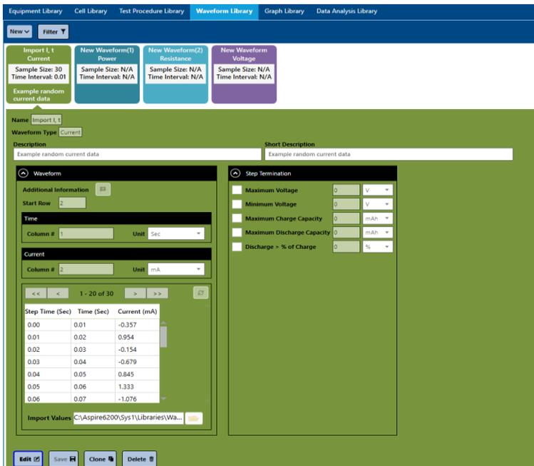
user to another). Each waveform has an individual library entry. Different colors are used to represent current, voltage, power, or load profiles as shown above. Unlimited numbers of waveforms can be stored.
