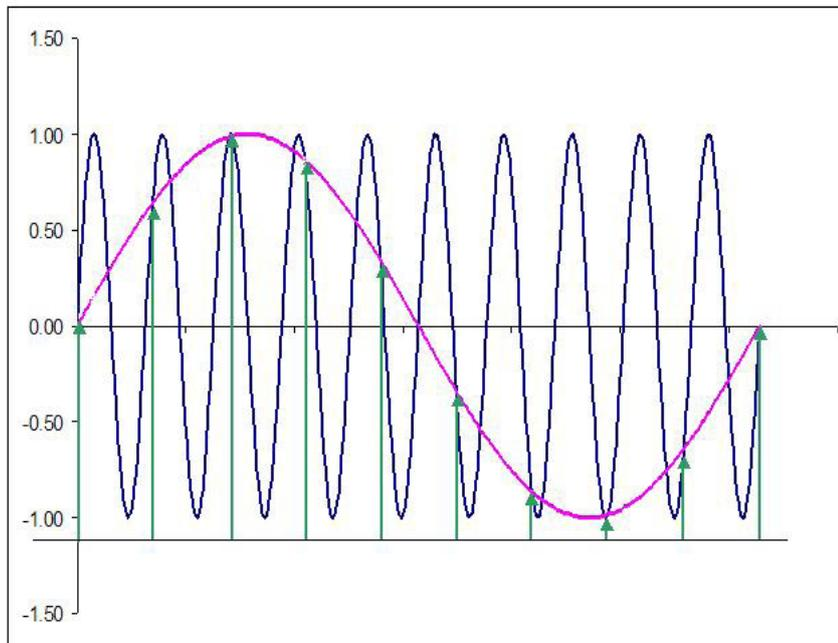
Figure 1: Sub-sampling a sine wave
