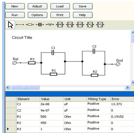
**Figure 11:** Equivalent Circuit Modeling tool. Elements can be selected from a drag and drop menu. The circuit shown in this figure was used to model the impedance response of the solar cell from 200 kHz to 100 Hz.
