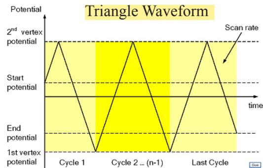
Figure 1 c Description of Potential Pulse Waveform. Normal, Differential and Square Wave options included
