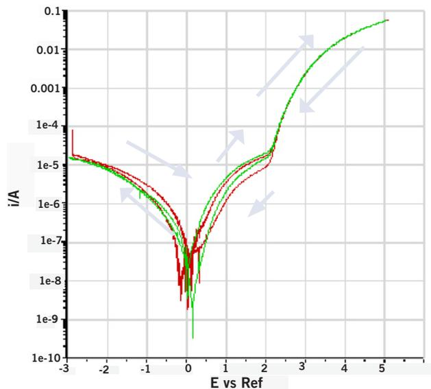
**Figure 2:** I-V curve of an OLED pixel as a function of scan direction (indicated by arrows) and scan speed. Green line =  $100 \text{ mV s}^{-1}$ , red line =  $300 \text{ mV s}^{-1}$ . Hysteresis indicative of charge trapping
