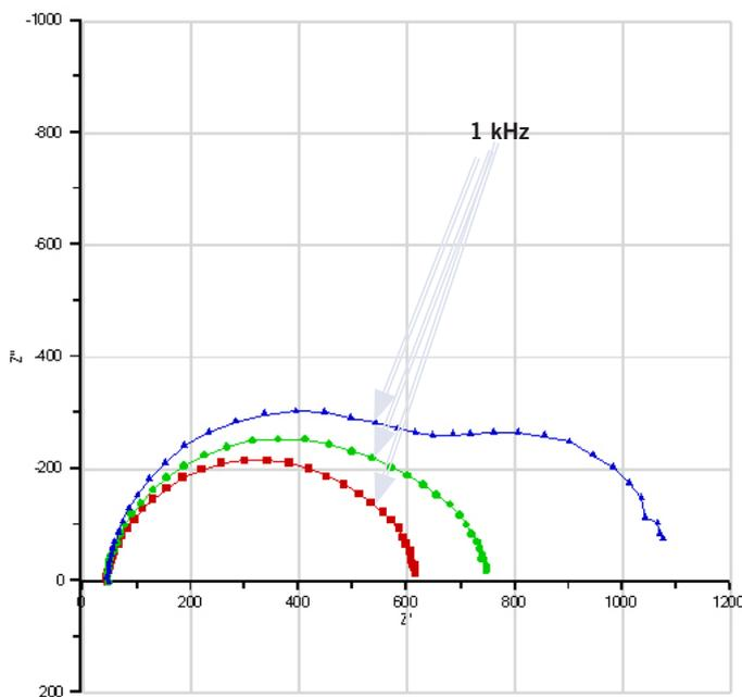
**Figure 10:** Nyquist / Cole-Cole diagrams of a solid-state solar cell under varying DC bias (note this experiment was performed under illumination). AC stimulus level was 100 mV.
