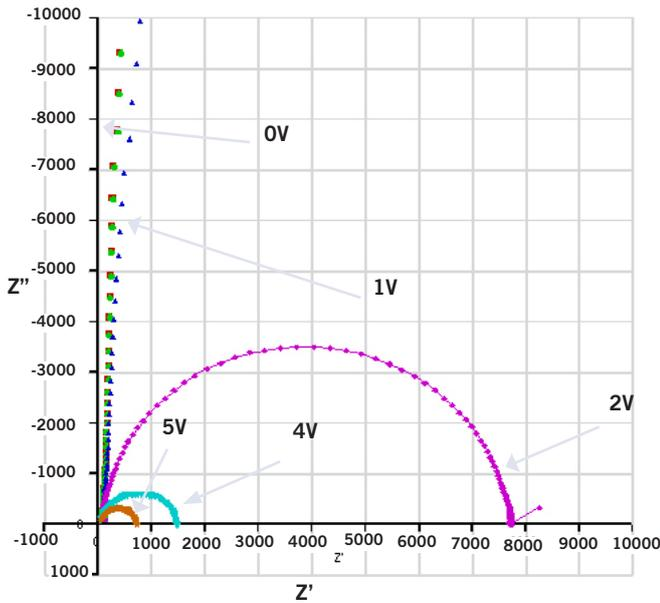
**Figure 4:** Cole-Cole (Nyquist) plot of the OLED operated under different DC bias voltages (as shown in the diagram)
