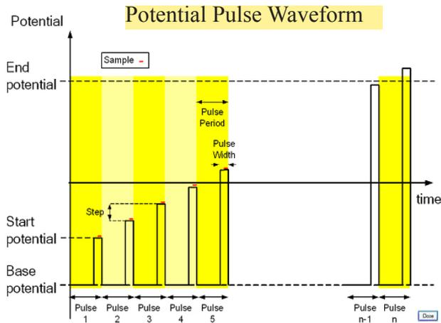
**Figure 2c** Potential pulse waveform. The user has the ability to define the pulse period, step height and pulse width. Minimum pulse width = 1  $\mu$ s
