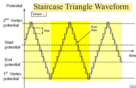
**Figure 2a and b** Description of a Triangle Voltage Waveforms (linear and staircase) for I-V characterization. Start, 1st vertex, 2nd vertex and end potentials are defined by the end user in the software. Multiple cycles can be used to determine cell stability. Scan rates from  $100 \text{ mVs}^{-1}$  to  $1 \text{ M Vs}^{-1}$  are available with data acquisition up to 1 Million samples per second.
