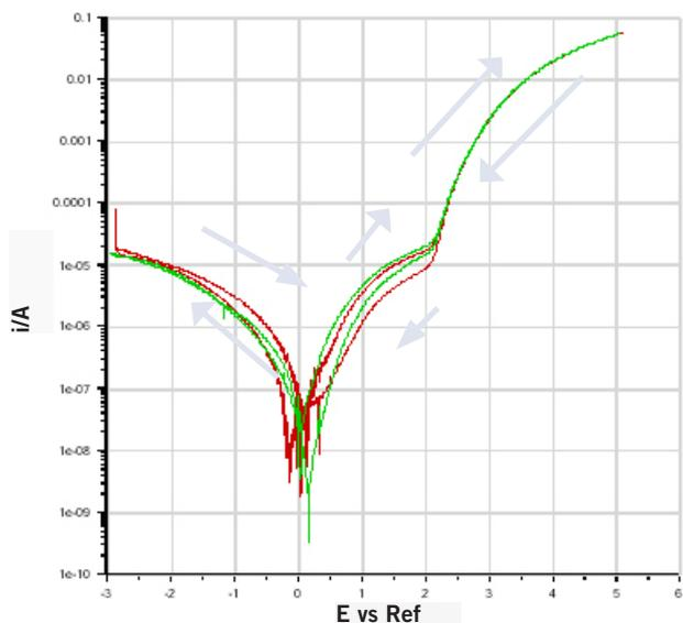
**Figure 1:** I-V curve of an OLED pixel as a function of scan direction (indicated by arrows) and scan speed. Green line =  $100 \text{ mV s}^{-1}$ , red line =  $300 \text{ mV s}^{-1}$ .
