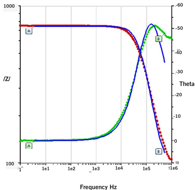
There are a number of alternative methods of presenting the impedance data which are supported in Solartron software including, Bode (Impedance, Phase vs. Frequency), complex capacitance and permittivity vs. Frequency, AC voltage and AC current vs. frequency. The use of these methods of data presentation are presented elsewhere in the literature but all have been shown to be useful in the development of our understanding of the fundamental electrical properties of the OLED.
