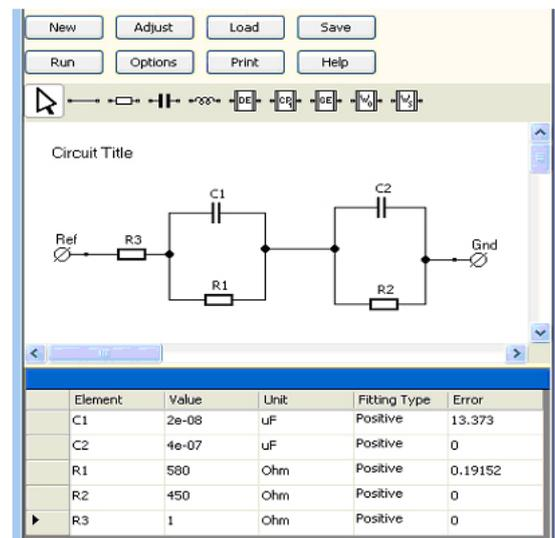
**Figure 6:** Equivalent Circuit Modeling tool. Elements can be selected from a drag and drop menu. The circuit shown in this figure was used to model the impedance response of the solar cell from 200 kHz to 100 Hz.
