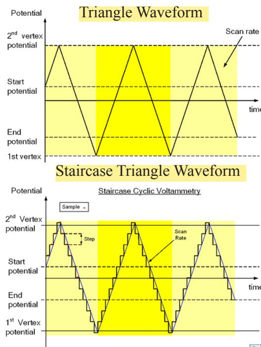
**Figure 2a and b** Description of a Triangle Voltage Waveforms (linear and staircase) for I-V characterization. Start, 1st vertex, 2nd vertex and end potentials are defined by the end user in the software. Multiple cycles can be used to determine if the system is stable under a varying load. Scan rates from  $100 \mu\text{Vs}^{-1}$  to  $1\text{M Vs}^{-1}$  are available with data acquisition up to 1 Million samples per second.
