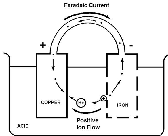
Corrosion rate proportional to Faradaic current
