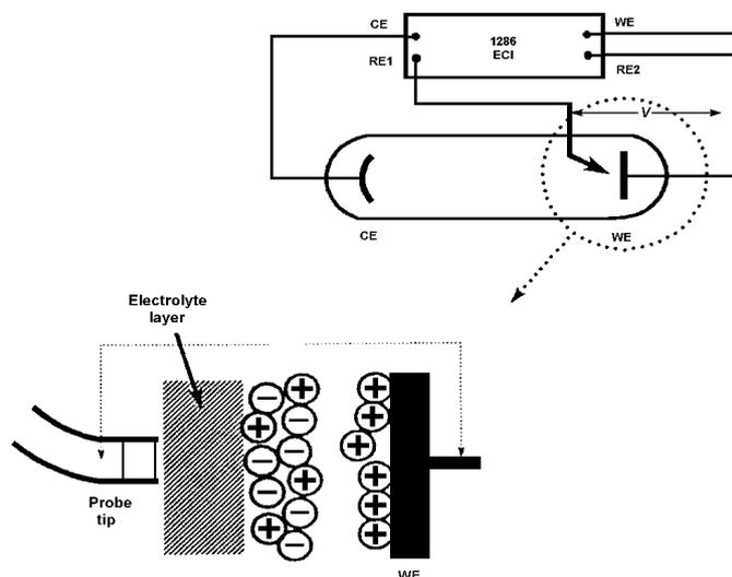
44. This layer of electrolyte has an unwanted resistance which is in series with the double layer. It is the **PARASITIC ELECTROLYTE RESISTANCE  $R_p$** . Voltage  $V$  includes the potential drop across  $R_p$  as well as the double layer.
