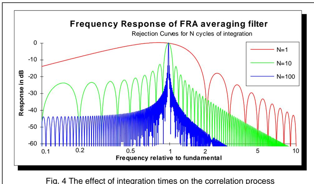
Fig. 4 The effect of integration times on the correlation process
