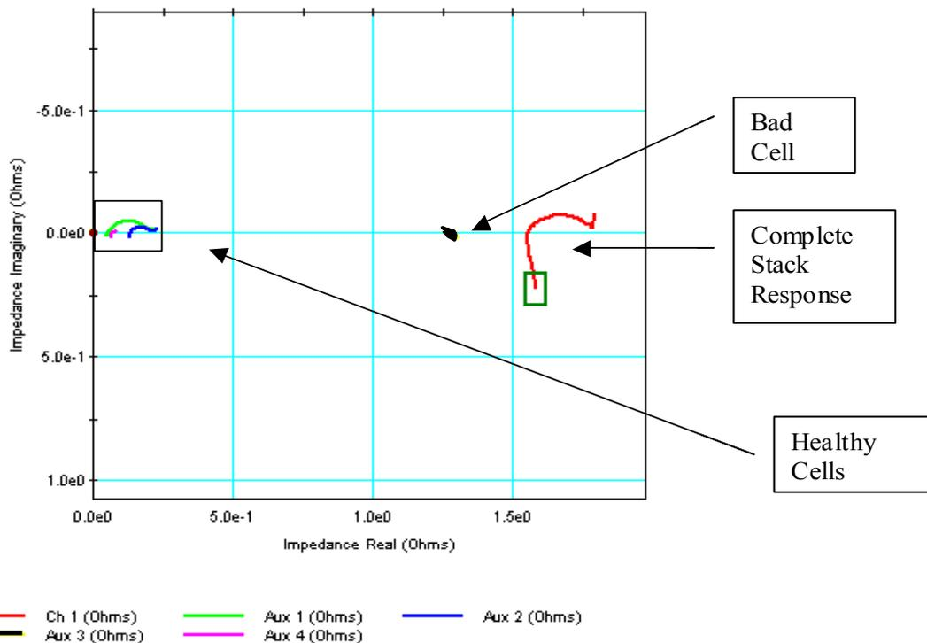
Figure 2: Complex plane plots of entire stack (red curve) and individual cells. FRA settings: single sine correlation with 1 second integration, AC stimulus = 20mA
