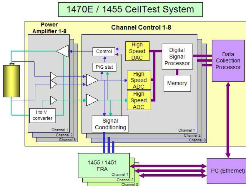
Figure 1: Block diagram of the CellTest multi-channel impedance test system
