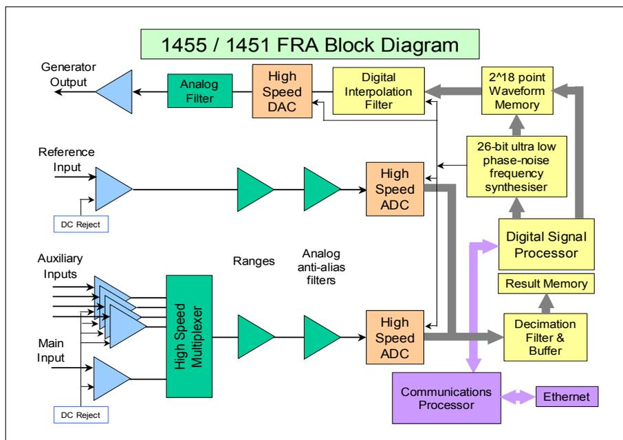
Figure 3: Block diagram of the 1455 / 1451 frequency response analyzer
