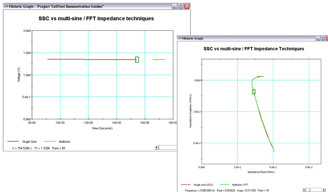
The single sine measurement is presented in red, multi-sine / FFT in green on the above plots. The impedance results are very similar although there is a little more noise associated with the multi-sine / FFT measurement, which is to be expected. The speed of multi-sine / FFT when compared with single sine is clearly shown on the time graph. Indeed, the measurement time was less than one fifth of that of the equivalent SSC measurement.
