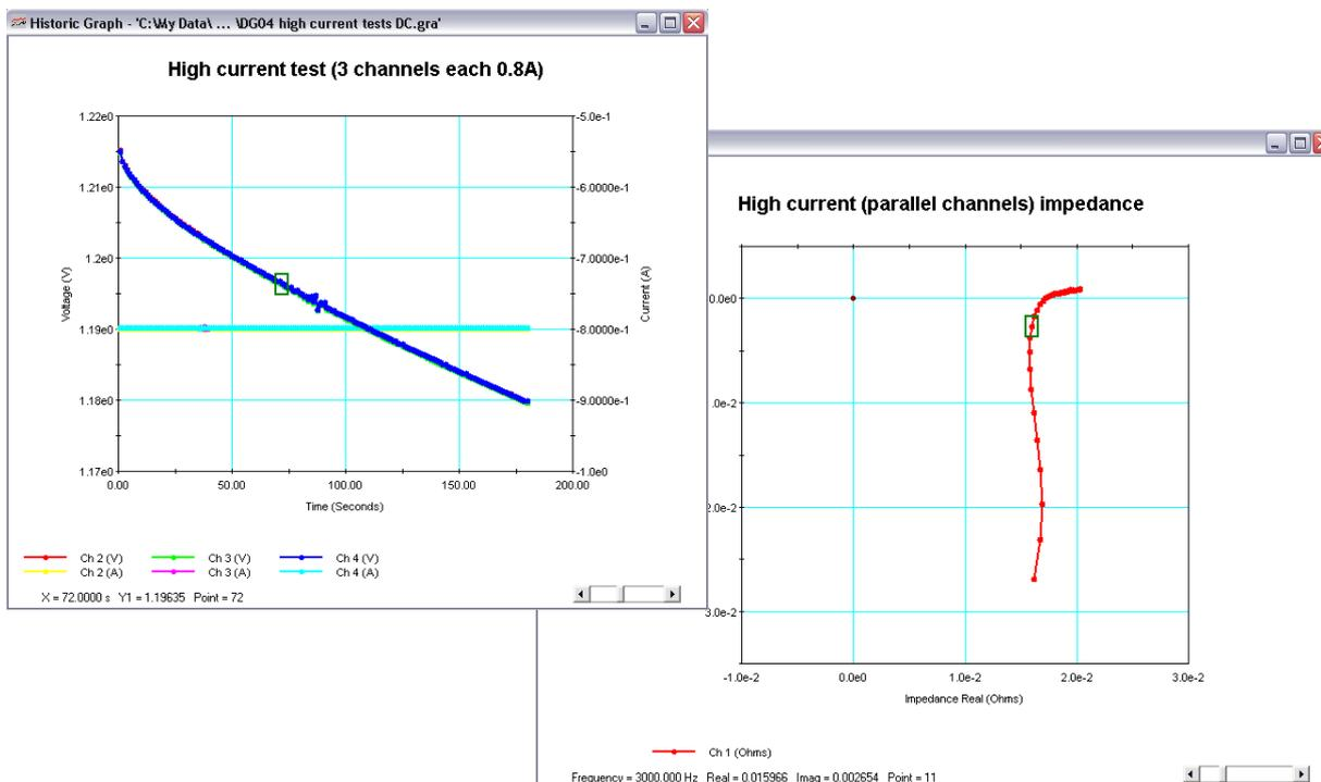
The DC results from channels 2-4 are shown (above left) confirming that each channel was discharged at 0.8 amps (the total discharge was therefore 2.4 amps from the four cells connected in parallel). The voltage measurements from these channels were overlaid on the same plot and this confirms that the cells were discharging (voltage reducing). The complex plane plot (above right) shows the impedance analysis from channel 1 which was measured during the cell discharge.
