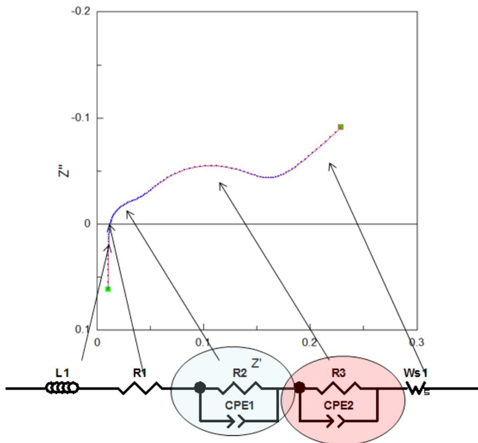
Figure 1: EIS results in Nyquist form from a Li-Ion battery at 100% SoC. The equivalent circuit model is used to simulate the EIS response of the cell. The circuit elements corresponding to the features in the EIS plots are shown. The data is modelled in the industry standard analysis platform ZVIEW. Note-  $R2$  is the charge transfer resistance -  $R_{ct}$  and  $R3$  is the Solid Electrolyte Interface Impedance -  $R_{sei}$
