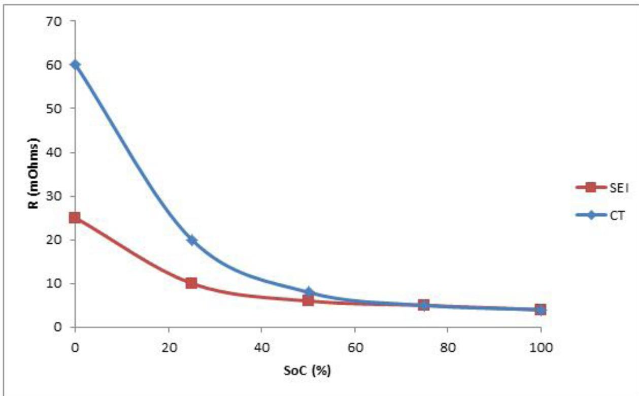
Figure 2: Impedance values calculated for circuit elements RCT and RSEI (Figure 1) as a function of SoC. Note how both values increase with decreasing SoC.
