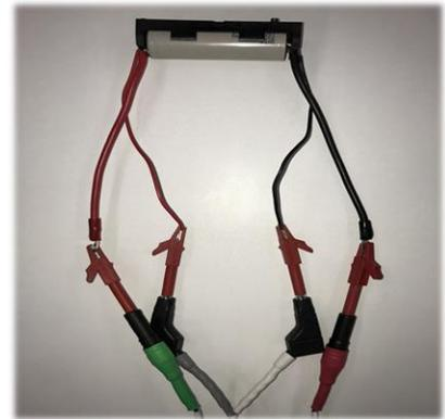
4T Connections to cell anode and cathode
