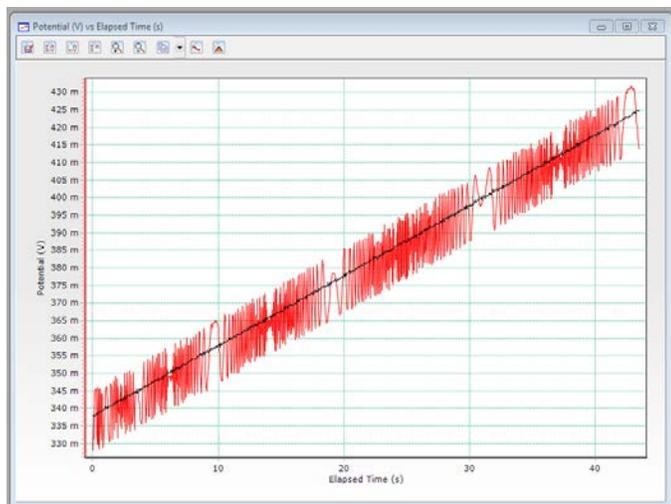
**Figure 7: Potential vs. time plot from Linear scan voltammetry of a 100  $\mu$ F capacitor in single-ended (black) and differential (red) mode**
