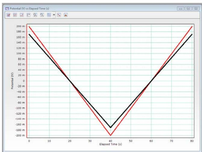
**Figure 5: Potential vs. time plot from cyclic voltammetry of a  $1\ \Omega$  resistor in single-ended (black) and differential (red) mode.**
