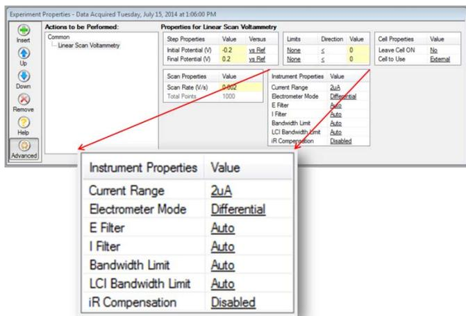
**Figure 1:** *Experiment Properties* window in VersaStudio showing the *Advanced* panel where the *Instrument Properties* settings can be selected.
