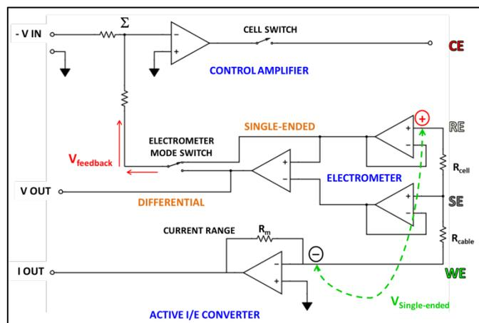
**Figure 4:** Potentiostat block diagram depicting contributions to the feedback voltage when measured in single-ended mode.
