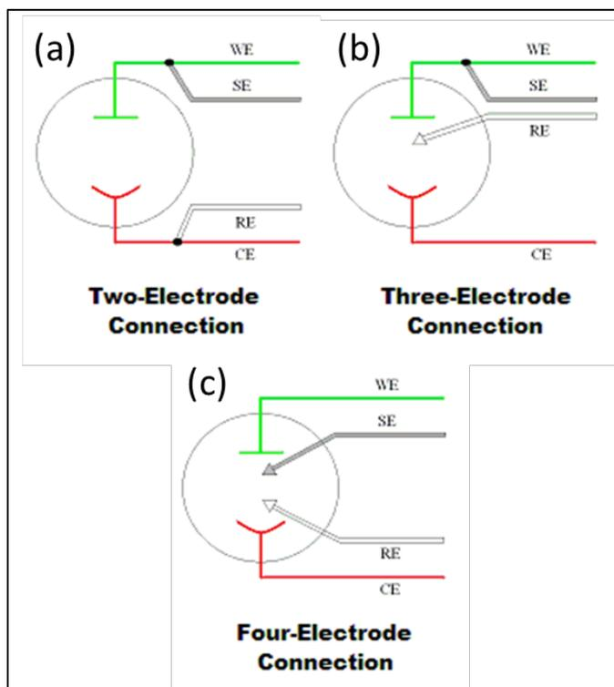
**Figure 3:** Schematic for two-, three- and four-electrode cell connections.
