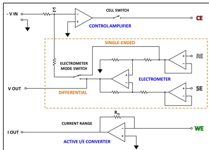
**Figure 2:** Potentiostat block diagram. V IN is the requested voltage and V OUT is the measured voltage recorded by the software. The dashed box encompasses the electrometer.
