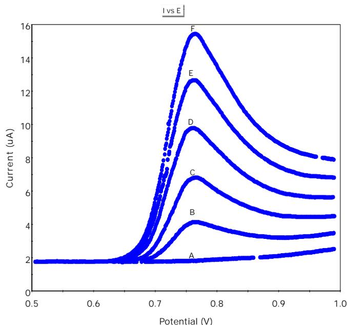
**FIGURE 20: Linear sweep voltammetry of butylated hydroxyanisole in 0.12 M H<sub>2</sub>SO<sub>4</sub> in 1:1 ethanol/benzene. A: Blank; B: 8.26 ppm; C: 16.4 ppm; D: 24.5 ppm; E: 32.6 ppm; F: 40.5 ppm.**
