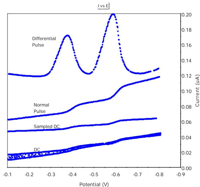
**FIGURE 11: Comparison of polarographic modes. 1 ppm  $\text{Pb}^{2+}$  and  $\text{Cd}^{2+}$  in 0.1M  $\text{HNO}_3$ .**
