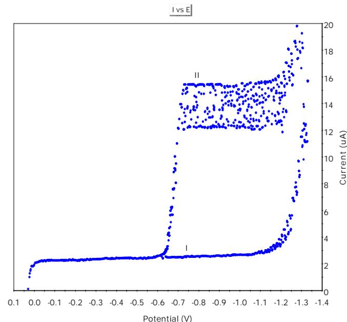
FIGURE 5: Polarograms of (I) 1M hydrochloric acid alone and (II) 1M hydrochloric acid containing 0.5 mM cadmium ion.
