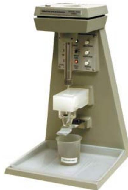
**FIGURE 2: PAR Model 303A Static Mercury Drop Electrode.**
