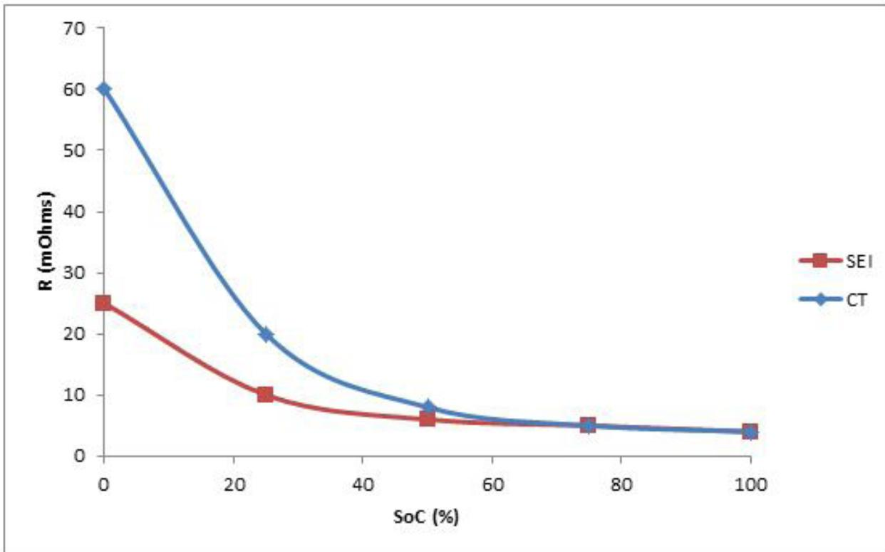
Figure 2: Impedance values calculated for circuit elements RCT and RSEI (Figure 1) as a function of SoC. Note how both values increase with decreasing SoC.
