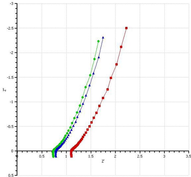
Figure 3: In-Stack Cell measurements for 3 Ni-MH batteries connected in series. The blue and green lines are the EIS responses of 'good cells' whilst the red line is an example of a 'bad cell'
