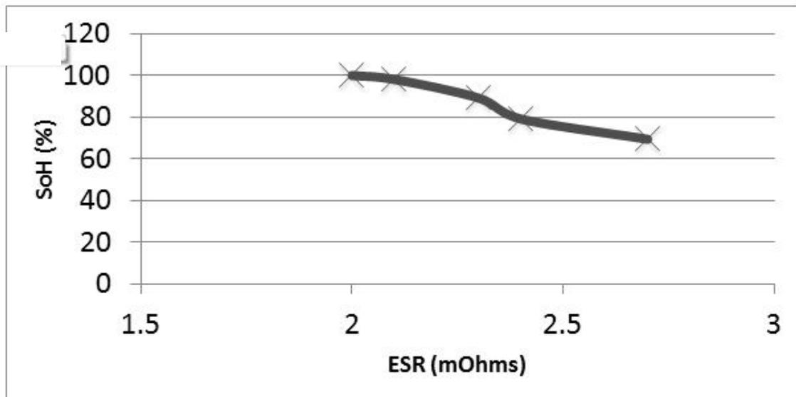
Figure 4: SoH (%) plotted vs the ESR (series resistance) of the cell as determined by analysis of the high frequency intercept from the complex plane / Nyquist plots.
