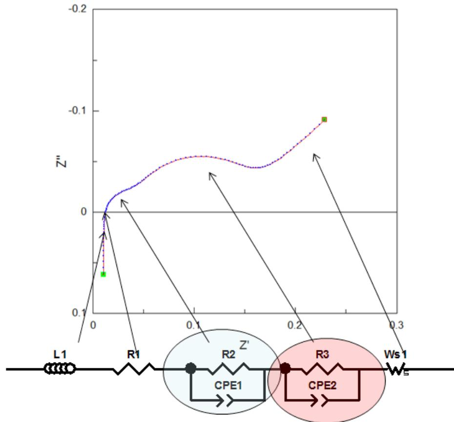
Figure 1: EIS results in Nyquist form from a Li-Ion battery at 100% SoC. The equivalent circuit model is used to simulate the EIS response of the cell. The circuit elements corresponding to the features in the EIS plots are shown. The data is modelled in the industry standard analysis platform ZVIEW. Note-  $R2$  is the charge transfer resistance -  $R_{ct}$  and  $R3$  is the Solid Electrolyte Interface Impedance -  $R_{sei}$
