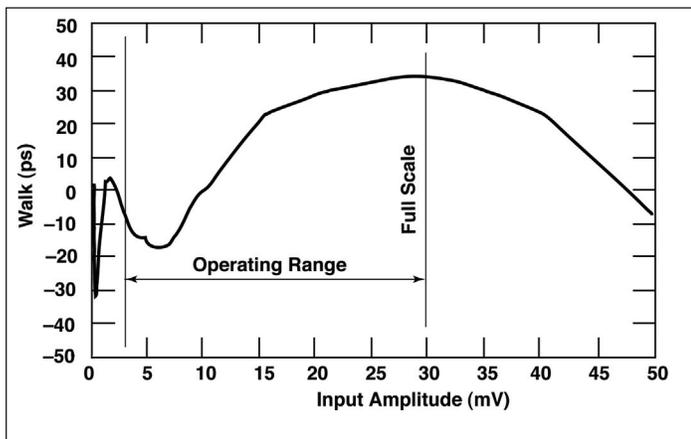
Fig. 3. Typical Walk vs. Pulse Amplitude. Full scale is denoted by the Over Range LED turning on. Measured with a pulse width of 300 ps FWHM.
