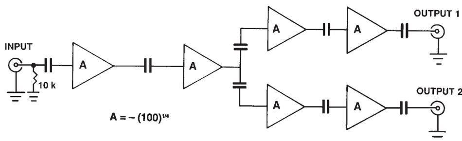
Simplified Functional Block Diagram of the Model 9306.
