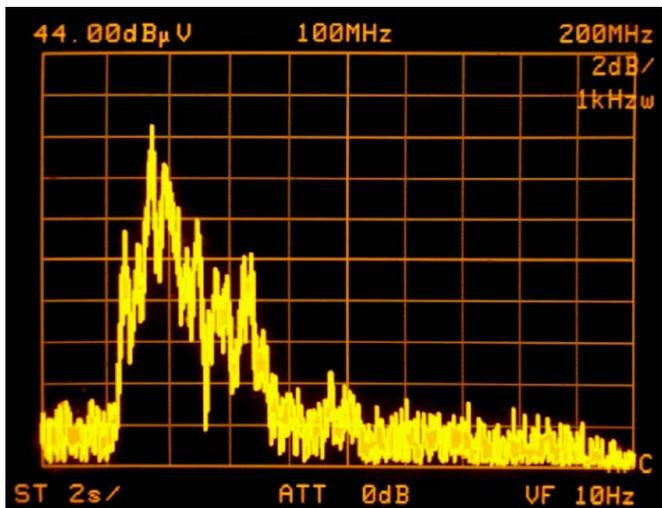
Figure 6, Background Spectrum when turned Off - Model 124A
