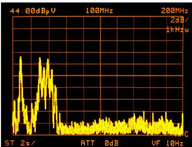
Figure 8, Background Spectrum when turned Off - Model 7124
