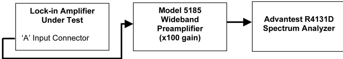
Figure 1, Spectral Measurement Test Setup
