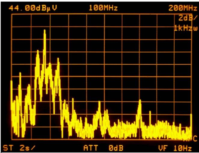
Figure 4, Background Spectrum when turned Off - Model 7265
