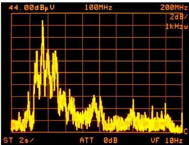
Figure 2, Background Spectrum when turned Off - Model SR830
