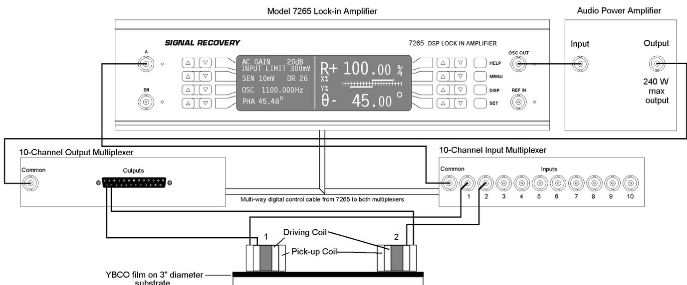
Figure 2, Ten-Channel System for Determining Critical Current Density in Superconductors
