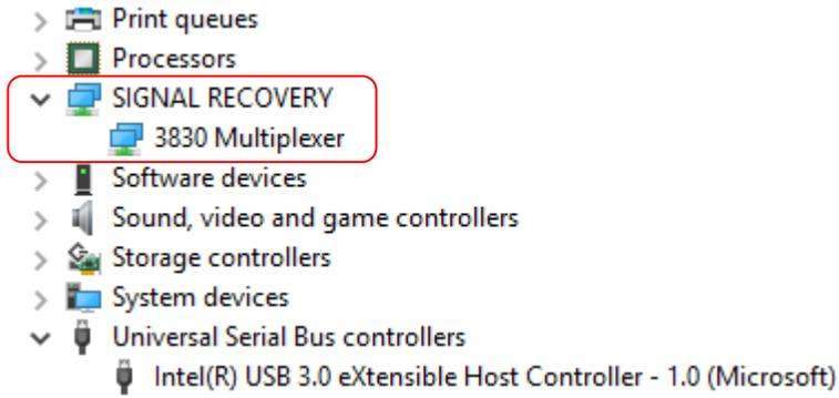
Figure 8, Device Manager (part listing), with 3830 Multiplexer Correctly Installed
