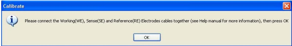
This configuration is shown below where the WE,SE, and RE are connected, but the CE is not. Once connected, select “OK” to continue.
