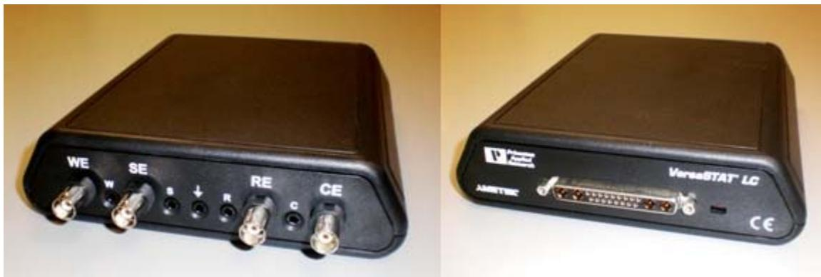
LCI Cell Cable Panel (left) and Potentiostat Interface Panel (right)
