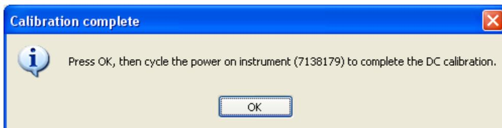
The calibration will not take effect until the system is re-booted by cycling the power on the potentiostat.
