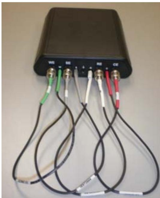
LCI with cell cables connected across internal feedback (dummy cell) resistor. The WE cable connects to the W pin jack, the SE cable connects to the S pin jack, the RE cable connects to the R pin jack and the CE cable connects to the C pin jack.
