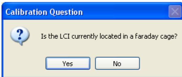
**NOTE: As the LCI is intended to measure ultra low currents, it is highly recommended that all experiments (and therefore, calibrations) be conducted in a shielded environment, such as a Faraday cage. Any experiments where nanoamps and lower are to be measured, a shielded environment must be used to block the electromagnetic fields that are prevalent in most all laboratory settings.**
