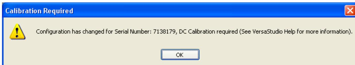
This message will appear after adding the LCI option to a system, as well as after removing the LCI option.
