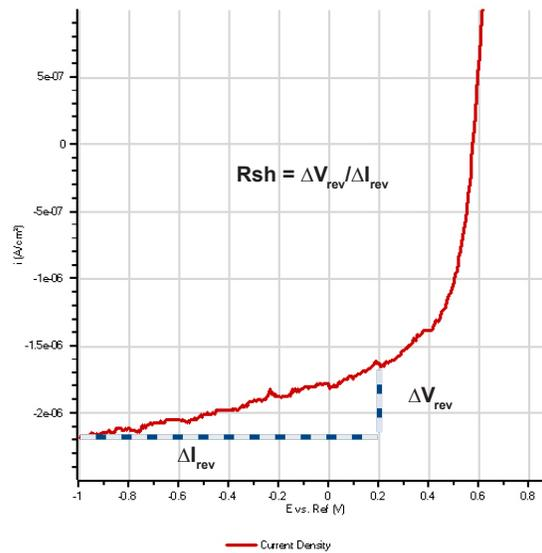
**Figure 3 :** Reverse Bias characteristics of an 18 V PV cell indicating method of calculating the shunt resistance. Analysis can be performed in software with regression tool. Note that for very low leakage current devices, Solartron systems have options to increase current resolution down to 0.15 fA.
