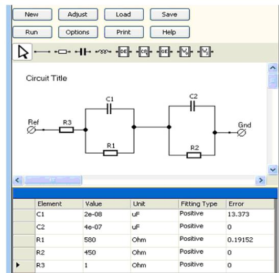
**Figure 6:** Equivalent Circuit Modeling tool. Elements can be selected from a drag and drop menu. The circuit shown in this figure was used to model the impedance response of the solar cell from 200 kHz to 100 Hz.
