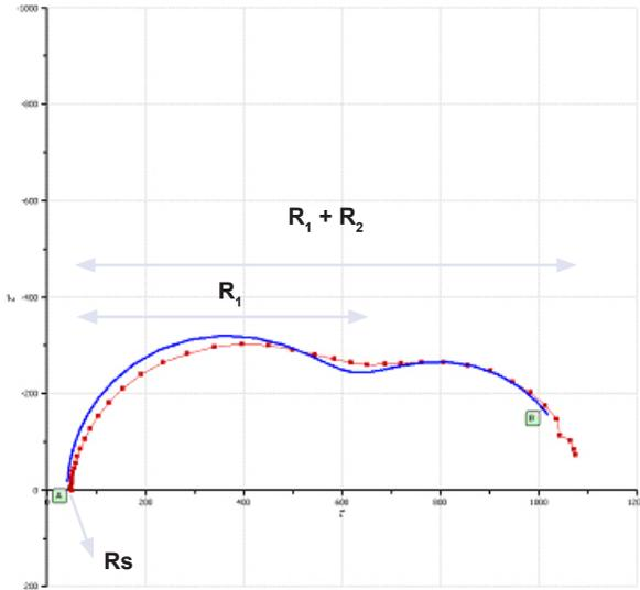
**Figure 7:** Comparison between the theoretical impedance response of the circuit shown in Figure 6 (blue line) vs. the real cell response (red line and dots). There is reasonable agreement between theory and experiment. The impedance values of  $R_1$  (contact) and  $R_2$  (recombination) are shown on the plot. In addition, the series resistance  $R_s$  can be calculated by determining the impedance at the point in which the high frequency measurement intercepts the real ( $Z'$ ) axis.
