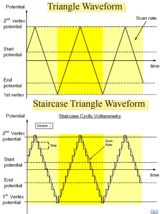
**Figure 2a and b** Description of a Triangle Voltage Waveforms (linear and staircase) for I-V characterization. Start, 1st vertex, 2nd vertex and end potentials are defined by the end user in the software. Multiple cycles can be used to determine if the system is stable under a varying load. Scan rates from  $100 \mu V s^{-1}$  to  $1 M V s^{-1}$  are available with data acquisition up to 1 Million samples per second.
